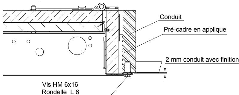
► **MONTAGE CONDUIT BETON POUR VOLET EI60S / EI90S – APL-13-A-845**
